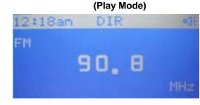
When pressed during normal play mode (XM/FM/AM/AUX/iPod), the audio output is muted or disabled as indicated by the speaker icon in the upper right corner of the display screen. When pressed again, the mute function is canceled and audio is restored. While the alarm is active, press this button to enter the snooze mode.
